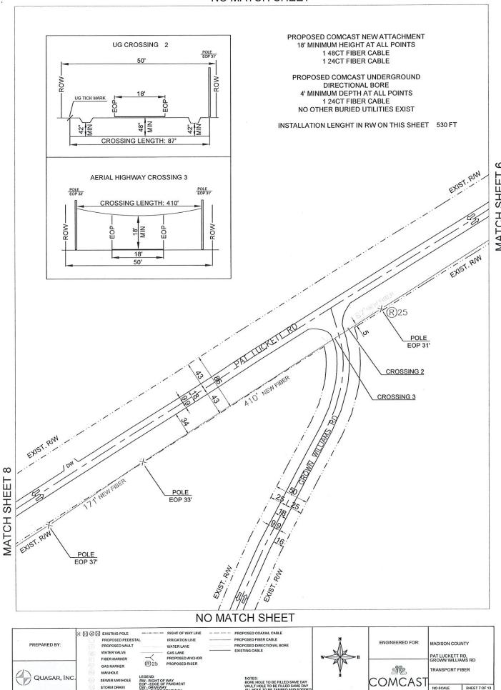
PROPOSED COMCAST NEW ATTACHMENT 18' MINIMUM HEIGHT AT ALL POINTS 1 24CT FIBER CABLE
